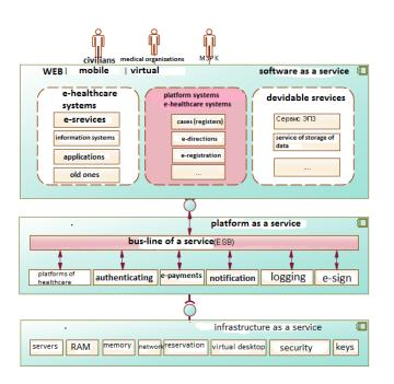
Figure 3. The architecture of cloud computing e-health.
