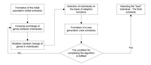
Figure 1. Scheme of the genetic algorithm
