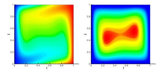
${\bf Figure 1.}$  Isotherms and stream lines of the problem of free convection when heated from the side
