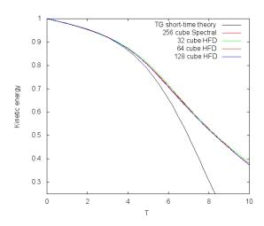
Figure 1. Comparison simulation result of the evolution of kinetic energy over the time with direct methods of Taylor - Green vortex at different Reynolds number
