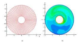
Figure 8. Estimated grid and the results of numerical solution of the temperature change
