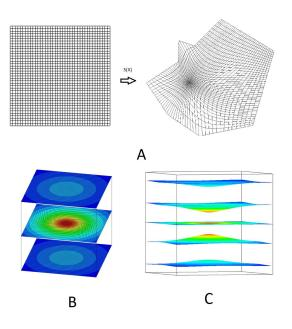
**Figure 1.** Structured grid construction: A) the mapping to be found; B-C) reverted Beltrami equation result.
