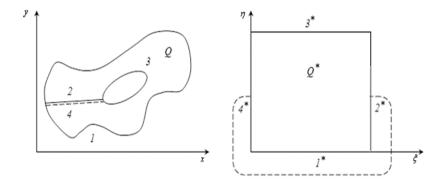
Figure 2. The mapping of a doubly-connected curvilinear domain Q to a calculated rectangle Q  $^\ast$
