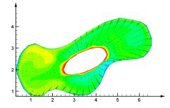
Figure 10. Results of the numerical solution of the temperature variation in the curvilinear domain
