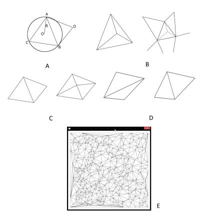
**Figure 2.** Delaunay triangulation: A) Delaunay principle; B) Delaunay construction: adding new point in triangular cell; C) Delaunay construction: adding new point to existing edge; D) flip operation; E) demonstration of constructed triangulation on the random 100 points.
