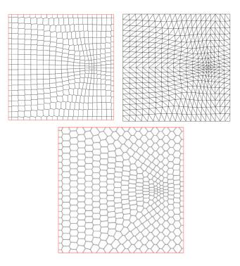
Figure 3. Example of unstructured grid constructed using points set defined by adaptive mapping: upper left and bottom – Voronoy diagrams and upper right – Delaunay triangulation.
