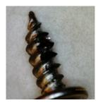
Figure 4. Defect - marks from tools.
