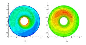
${\bf Figure 9.}$  The results of a numerical solution of a) temperature change, b) the current function at the same time
