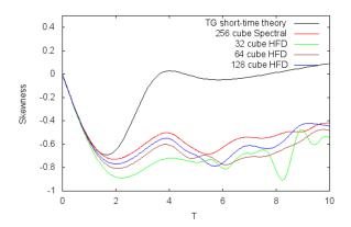
Figure 3. Comparison simulation result of the evolution of skewness over the time with direct methods of Taylor - Green vortex at Re=300
