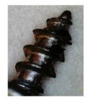
Figure 3. Defect - folds.
