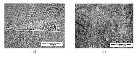
Figure 1. Microstructure of the studied samples of Grade 5 alloy Eli with ideal texture (a) and damaged texture (b).
