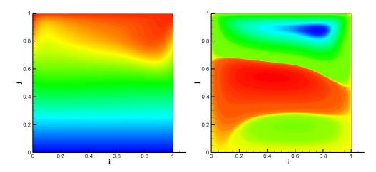
Figure 2. Isotherms and streamlines at Re = 500
