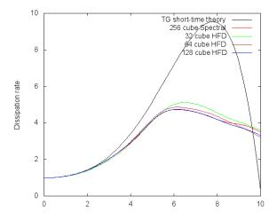
Figure 2. Comparison simulation result of the dissipation rate of turbulence decay over the time with direct methods of Taylor - Green vortex at different Reynolds number.
