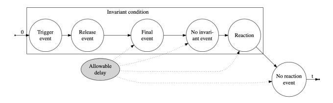
Fig. 1. A concept of specification for event-driven control requirements [13]
