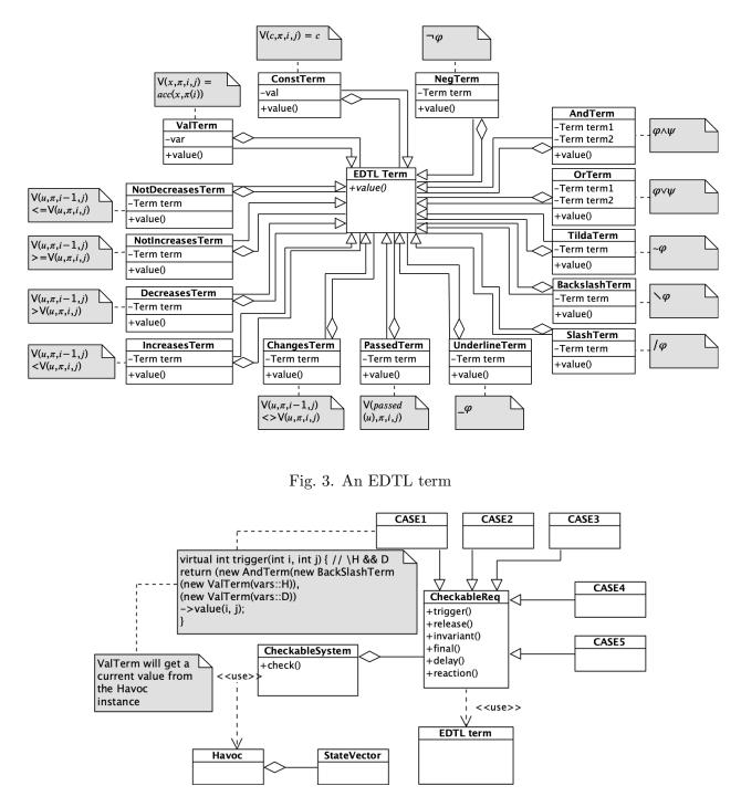
Fig. 4. A model of system with sets of requirements in the form of EDTL-terms
