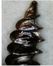
**Figure 1.** Defect of the implant carving in the form of a fracture.
