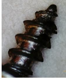
**Figure 3.** Defect - folds.
