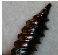
**Figure 5.** Defect is a flash.
